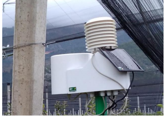
Figure 4. Sensor node for measuring air quality parameters.
